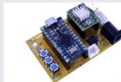
The core of this device. This PCB will control the stepper motor. Configurable for any DIY StarTRACKER via Arduino CODE
